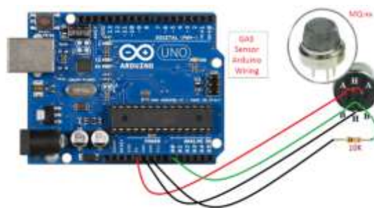
Fig -3: Gas sensor with Arduino board
