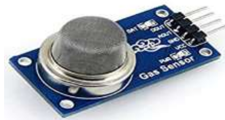
Fig -2: Gas sensor
