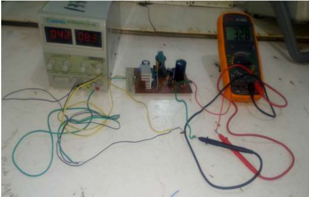
Fig. 4: Complete Circuit Prototype Showing DC Voltage Input And Output
