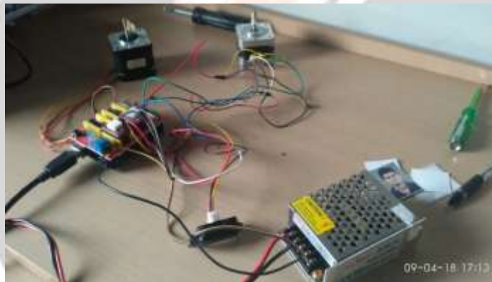
Fig.5 Arduino, stepper motor and Power supply of 3D scanner.
