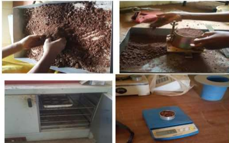
Fig-7: Standard proctor compaction test for soil-cement mix
