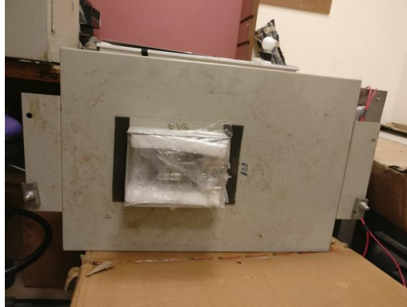
Fig 5 : Back Side of PIB box with simple clamps
