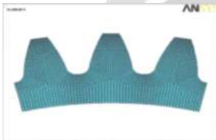
Figure 4 :Finite element Model of three teeth gear segment with profile -2 fillet
