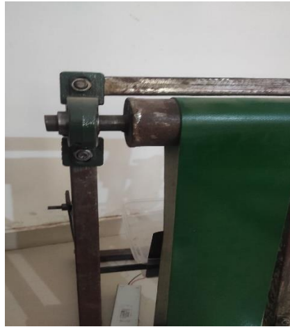
Fig.6.Adjustment for changing belts
