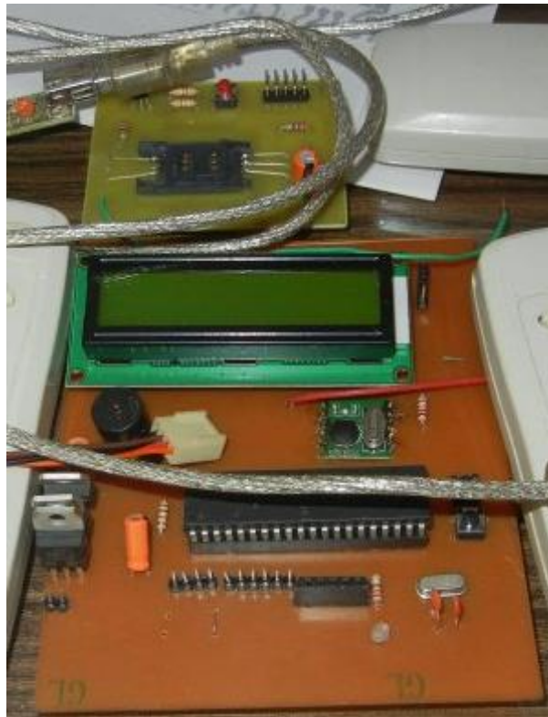
Fig.2 shows the Internet(GSM) Receiver Module
