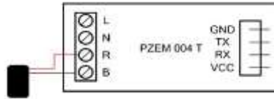
Figure 3. Schematic diagram of PZEM 004T
