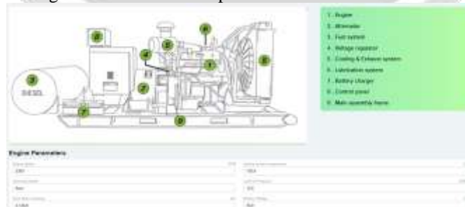
Fig. 3. Smart Diesel generator (6).
