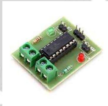
Fig 3. L293D Motor driver
