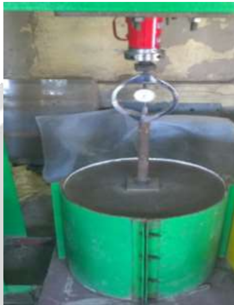
Figure-1: Setup for model Plate load test
