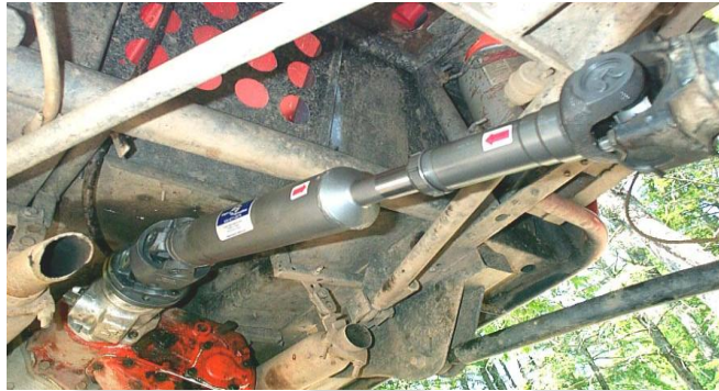
Fig-4: A Two-Section Drive Shaft of a Truck
