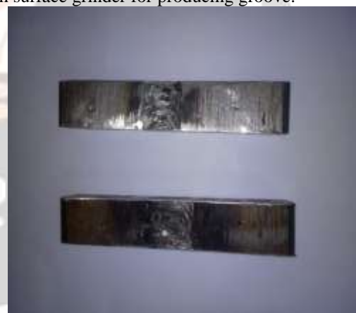
Figure 3.2: Cutted specimen of AISI 304 with coating (62mm×10mm×10mm)
