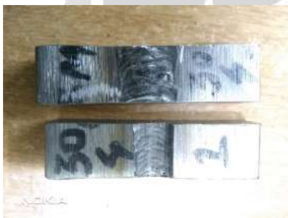
Figure 3.1: Cutted specimen of AISI 304 without coating (62mm×15mm×15mm)
