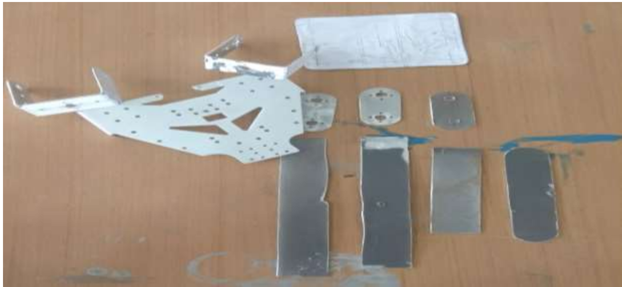
Figure 2.1. Part manufacture in work shop (aluminum) bracket
