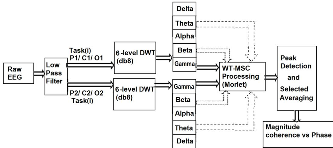
Fig.-6 Block diagram of processing steps for MSC and phase synchronization analysis
