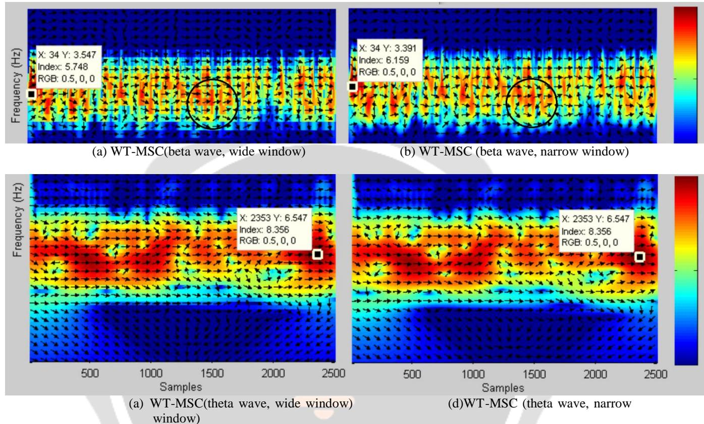
Fig.-5: Impact of Fourier window size on spectral power (magnitudes are in db)
