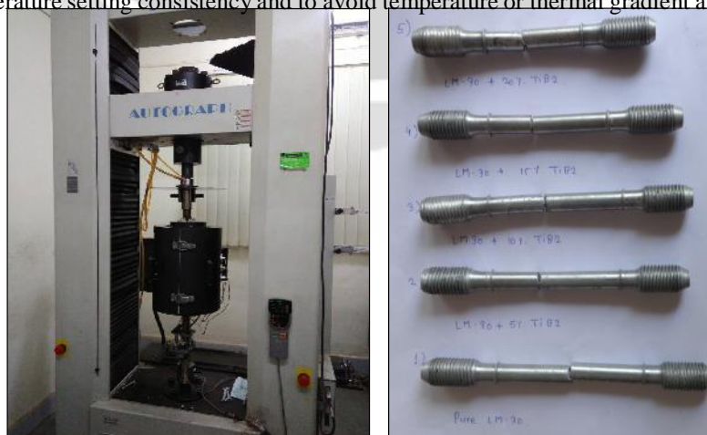
Fig -2: Hot Tensile Test Setup (SHIMADZU) & Actual Breaking of Sample
