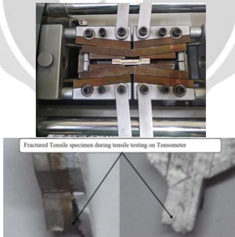
Figure 6. Tensile specimen (a) placed in the Tensometer for tensile testing (b) Fractured specimen after completion of the process of tensile testing
