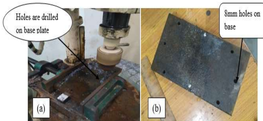
Figure 2. (a) Drilling on the base material, (b) Drilled base
