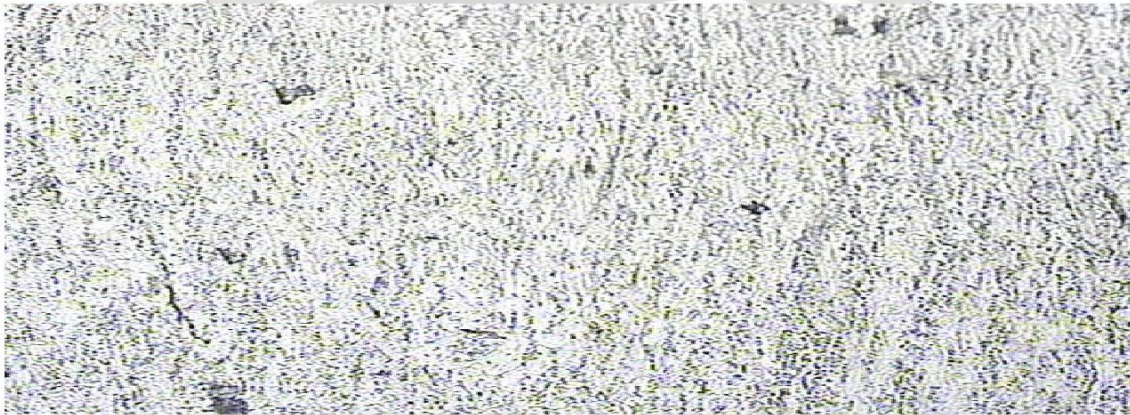
Fig. 12: Core Microstructure of Nitrided Specimen Nital 3 % 100
