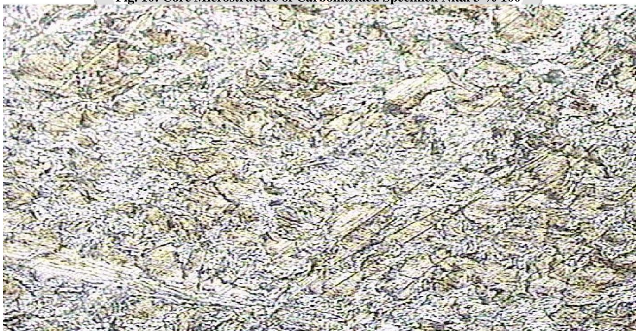
Fig. 11: Core Microstructure of Carbonitrided Specimen Nital 3 % 500 X
