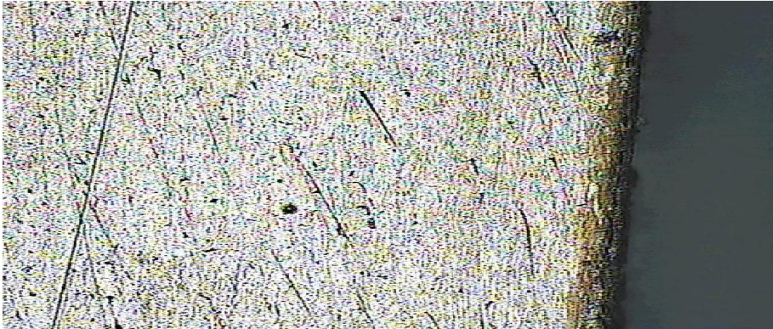
Fig.11: Case Microstructure of Nitrided Specimen Nital 3 % 100 X
