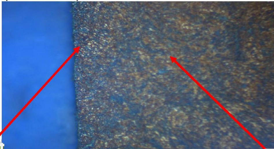
Fig. 6: Microstructure of SAE 1117 Carburised & Hardened Specimen Nital 3% 100X
