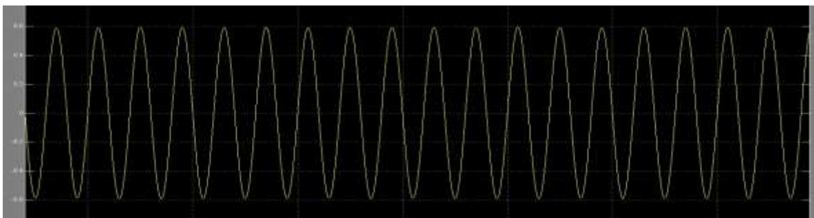
Fig.6 Grid Side Current Waveform
