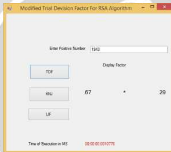
FIGURE 1: THIS WINDOW SHOW THAT IN INPUT BOX WE GIVE 1943 INPUT VALUES AND HIT THE TDF METHOD BUTTON OF MODIFIED TRIAL DIVISION FACTOR FOR RSA ALGORITHM AND GET EXECUTION TIME IN MICRO-SECONDS.
