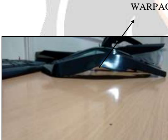
Fig.5 Initial Belly Pan with warpage and other defects
