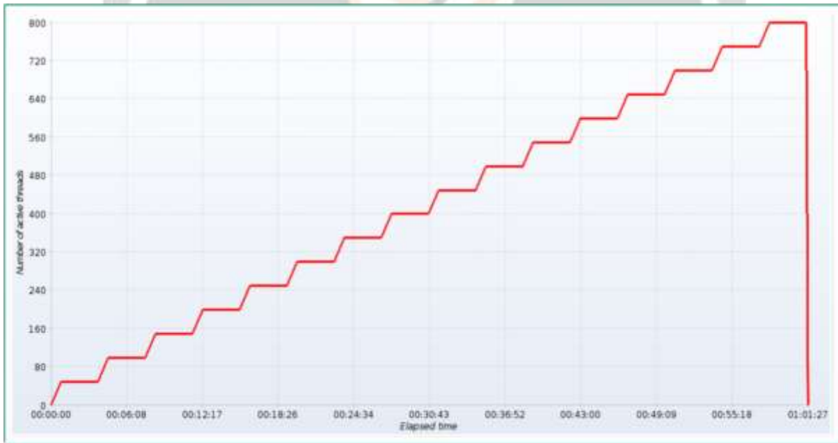
Figure 8 Graph of Number of threads v/s elapsed time for average load predefined step size.
