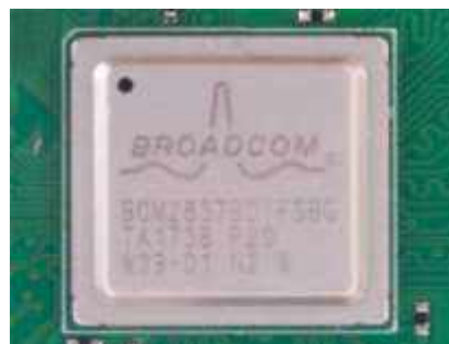
Fig -2 The heart of the Raspberry Pi 3 Model B+
