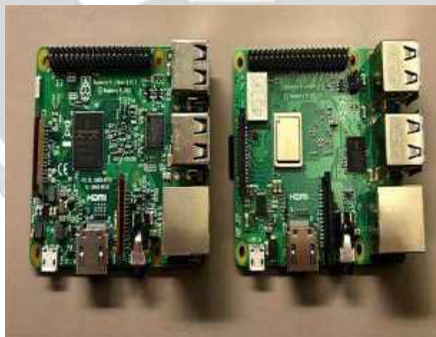
Fig -4 Comparison of the Raspberry 3 and 3 B+
