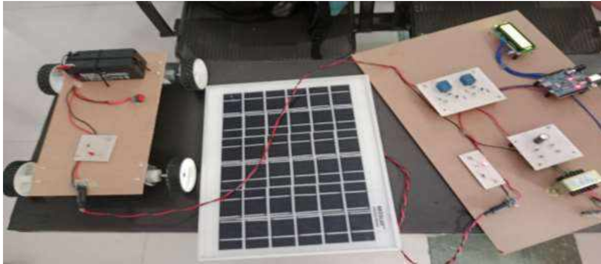
Fig6.Our EV Charging system
