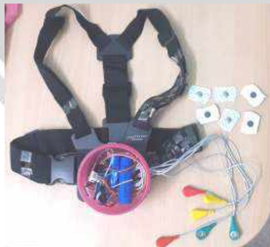
Fig -1: Complete Wireless ECG Monitoring apparatus
