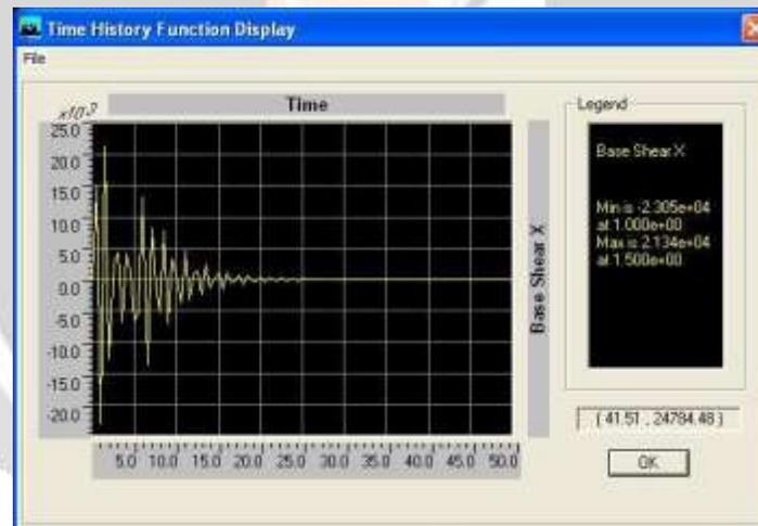
Fig: 5 The Graph Showing between Time Vs Base shear X ( With TMD)
