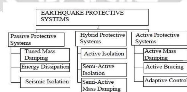
Fig. 1. General diagram of Earthquake protective system
