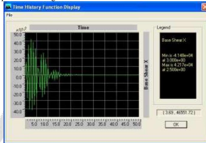
Fig: 4 The Graph Showing between Time Vs Base shear X ( Without TMD)
