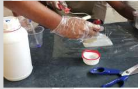
Fig-3 : Removing air using roller
