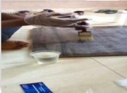
Fig-2 : Applying resin on mould
