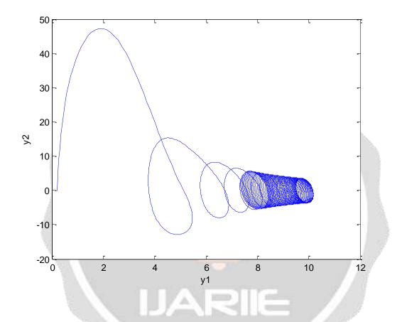
Graphical representation of the approximate solution of fractional order modified version of real fractional order the Van Der Pol Oscillator.
