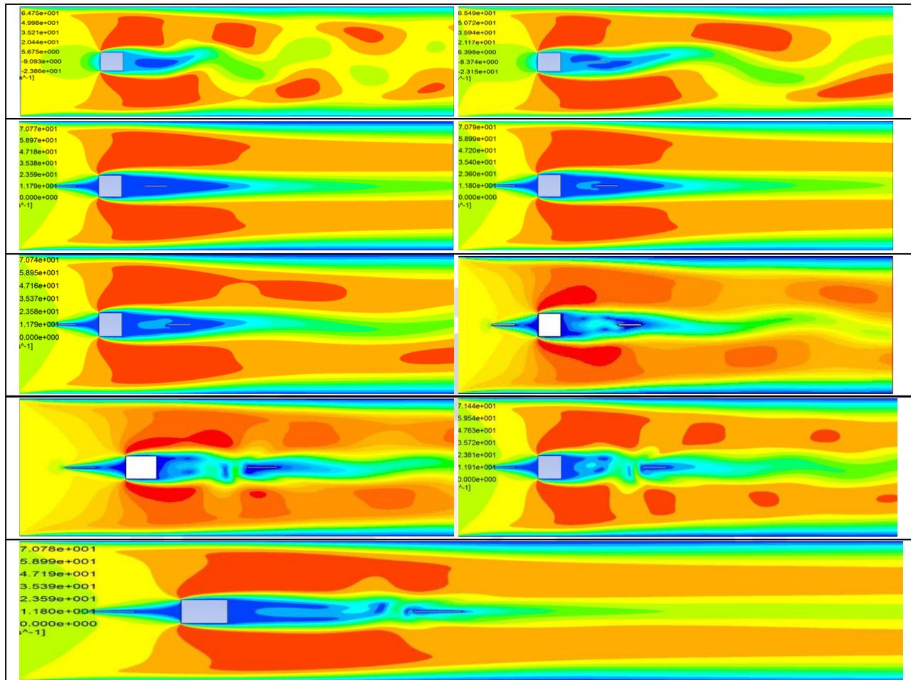
**Figure 3:** Velocity magnitude contours of square cylinder with detached plate at varying gap distances
