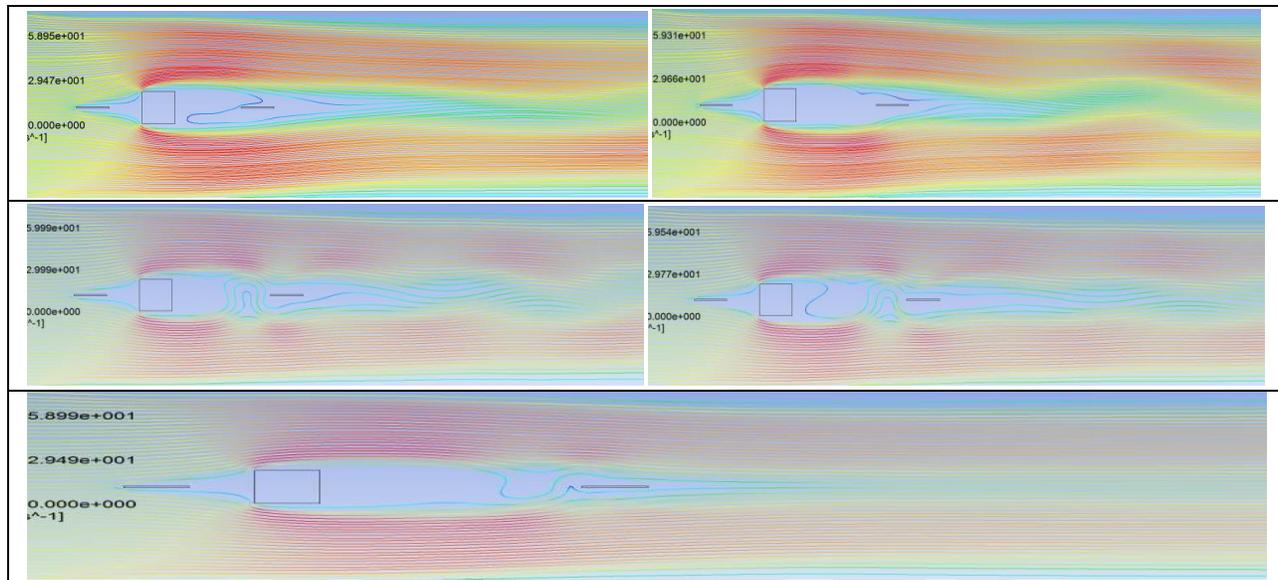
**Figure 4:** Streamlines contours of square cylinder with detached plate at varying gap distances
