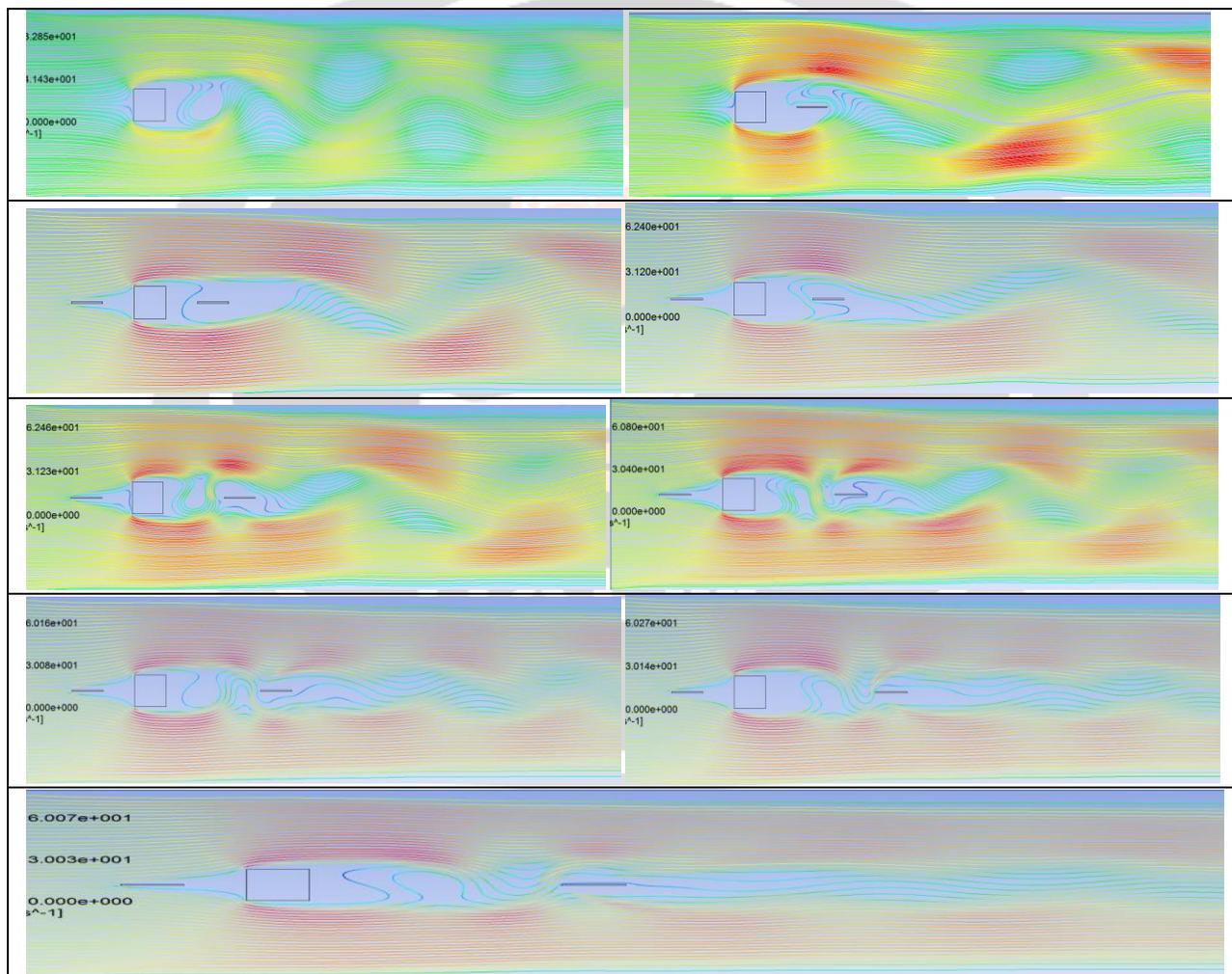
**Figure 6:** Streamlines contours of square cylinder with detached plate at varying gap distances
