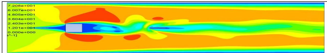
**Figure 5:** Velocity magnitude contours of square cylinder with detached plate at varying gap distances
