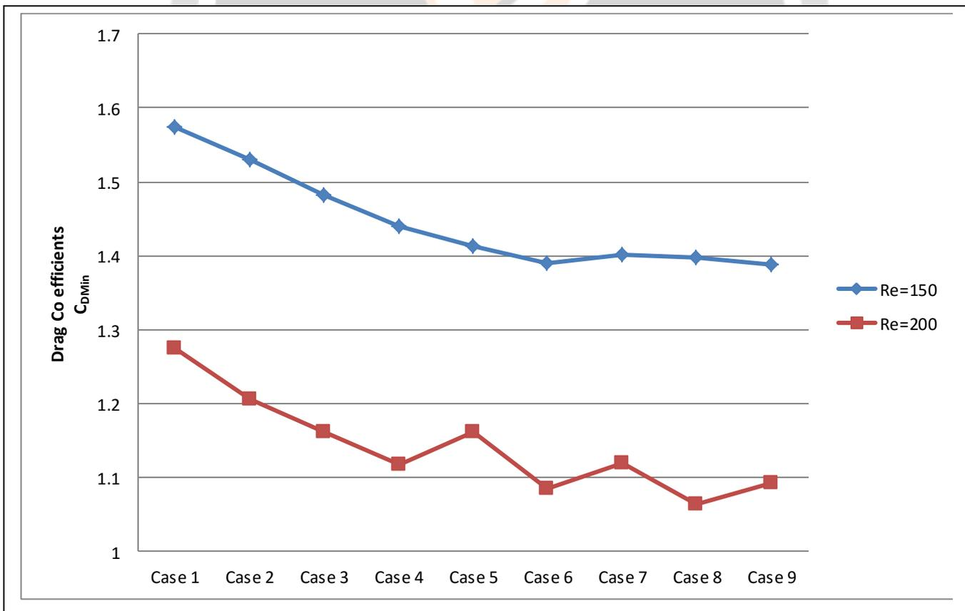
Figure 8: Coefficient of drag variation for varying gap distances
