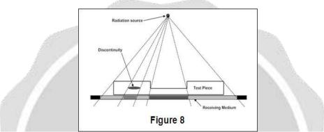
Industrial radiography involves exposing a test object to penetrating radiation so that the radiation passes through the object being inspected and a recording medium placed against the opposite side of that object. For thinner or less dense materials such as aluminum, electrically generated x-radiation (X-rays) are commonly used, and for thicker or denser materials, gamma radiation is generally used.
