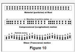
Compression waves cause the atoms in a part to vibrate back and forth parallel to the sound direction and shear waves cause the atoms to vibrate perpendicularly (from side to side) to the direction of the sound. Shear waves travel at approximately half the speed of longitudinal waves.
