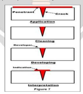
When performing a PT inspection, it is imperative that the surface being tested is clean and free of any foreign materials or liquids that might block the penetrant from entering voids or fissures open to the surface of the part. After applying the penetrant, it is permitted to sit on the surface for a specified period of time (the "penetrant
