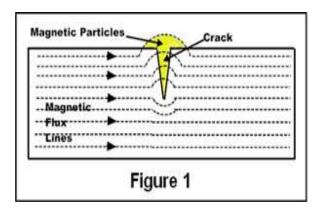
Because magnetic flux lines don't travel well in air, when very fine colored ferromagnetic particles ("magnetic particles") are applied to the surface of the part the particles will be drawn into the discontinuity, reducing the air gap and producing a visible indication on the surface of the part. The magnetic particles may be a dry powder or suspended in a liquid solution, and they may be colored with a visible dye or a fluorescent dye that fluoresces under an ultraviolet ("black") light.
