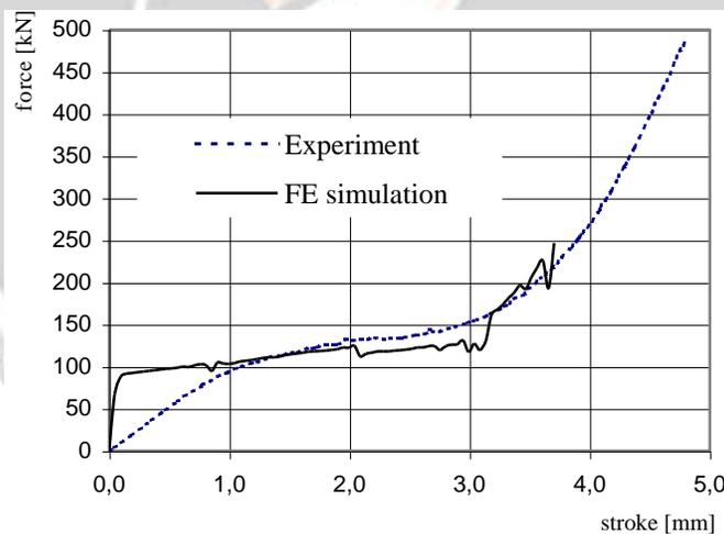
Fig. 4. Force-stroke diagram. Experiment (solid line), FE simulation (dashed line)
