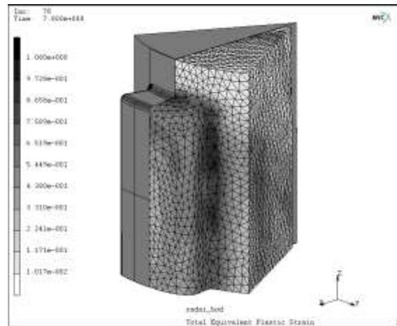
Fig. 1. Distorted body mesh of tetrahedral, four noded elements. Satisfactory fulfilment of gear cavity.
