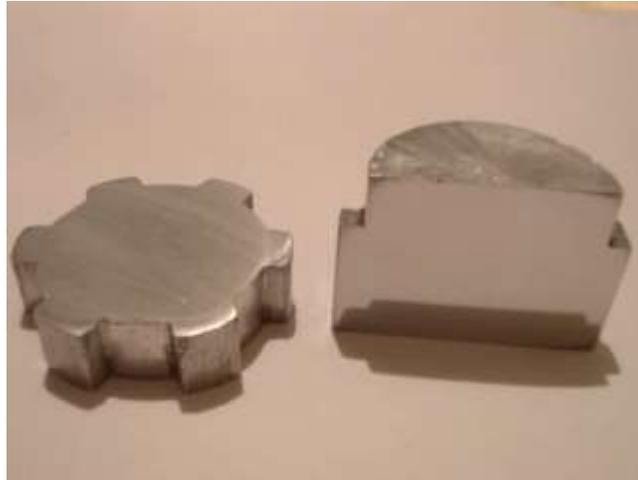
Fig. 3. Al billet cut in the horizontal and vertical planes in order to measure the microhardness using HV5.
