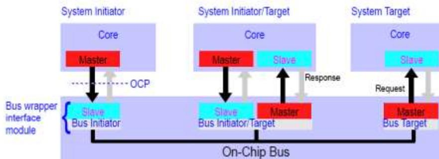
Fig. 1. Basic block diagram of OCP instance. [8]
