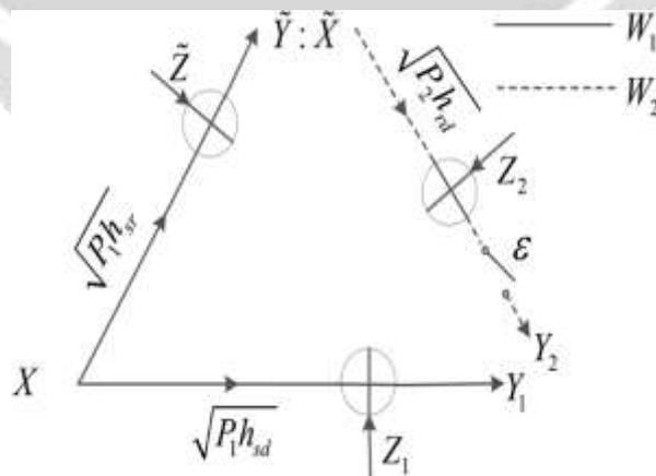
Fig.2 Heterogeneous cognitive Gaussian relay channel (HCGRC) model.
