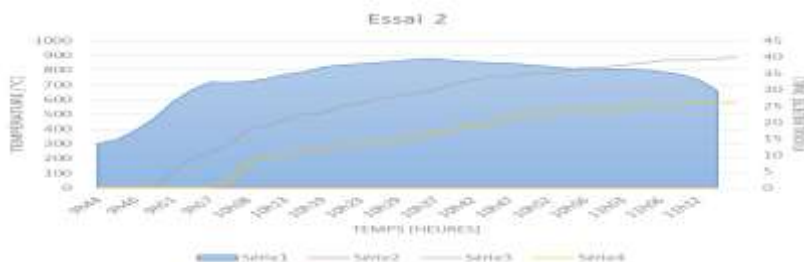
Figure 8: Curve of the evolution of emissions as a function of temperature and time (Test 2)
