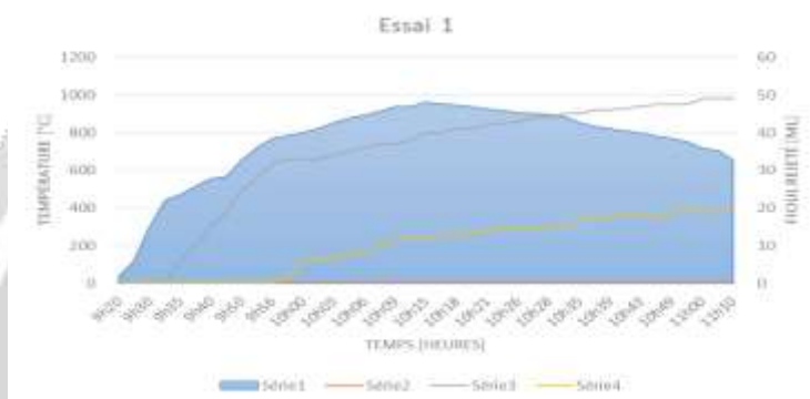
Figure 7: Curve of the evolution of discharges as a function of temperature and time (Test 1)
