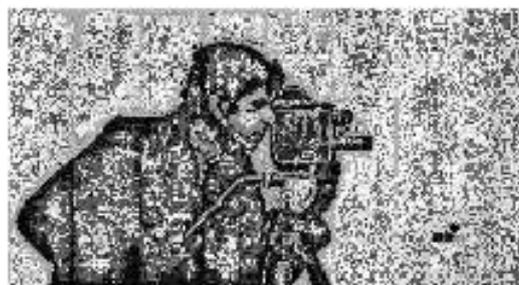
**Fig -23:** Received image if no amplifier linearization technique is used (SNR = 6dB)
