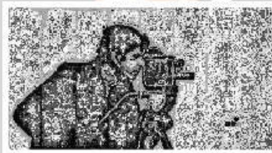
**Fig -27:** Received image if no amplifier linearization technique is used (SNR = 8dB)
