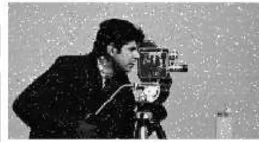
**Fig -25:** Received image after neural network-based predistortion (SNR = 6dB)
