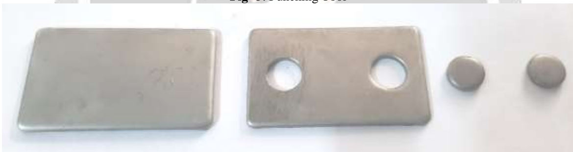
Fig -6: Step wise procedure of blanking and punching
