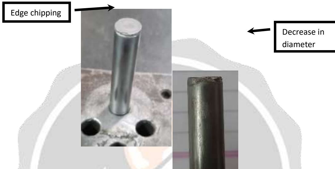
Fig -14: Wear on Punching Tool
