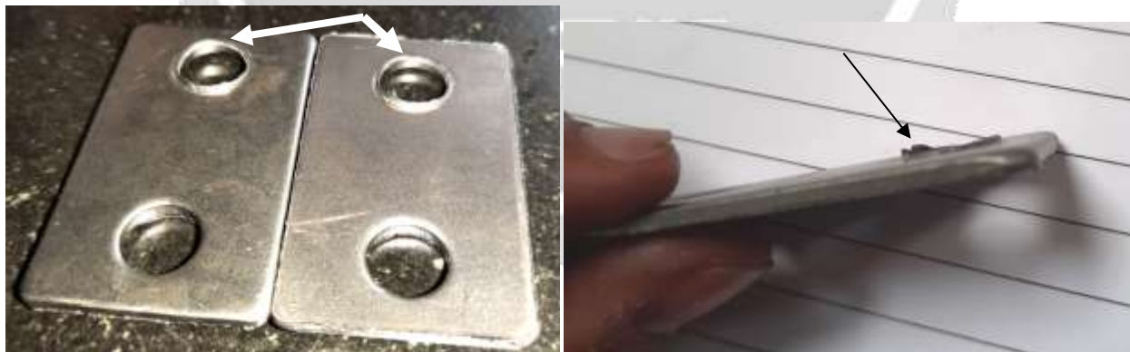
Fig -10: Heavy Burr on Bracket after Punching
