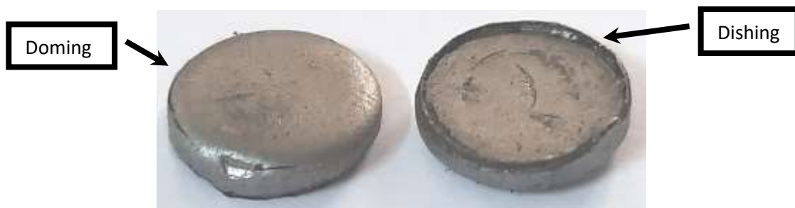
Fig -13: Dishing and Doming
