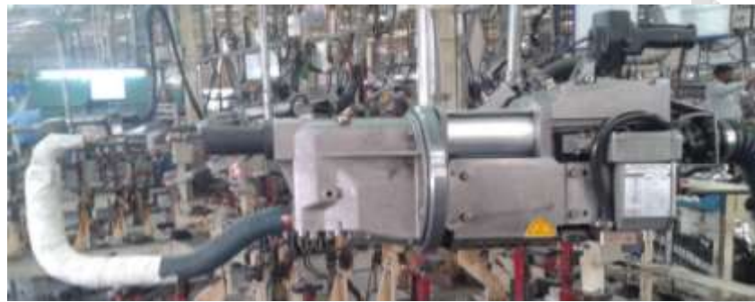
Fig-2 Integral Transformer Resistance Spot Welding Machine
