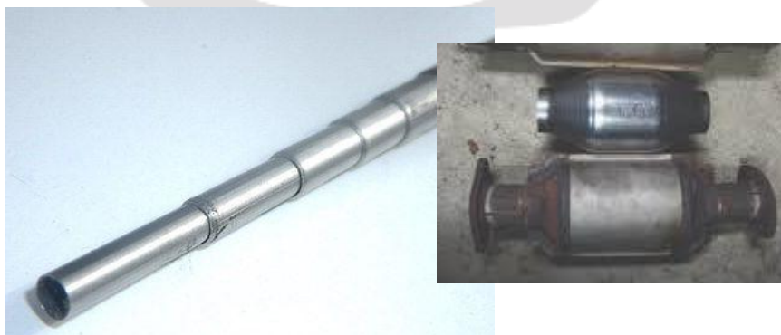
Figure.3 Photographic View of Telescopic Pipe and Catalytic converters used
