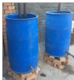
Fig -4 : Condenser of the pyrolyzer prototype
