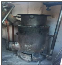
Fig -4: Pyrolyzer prototype reactor
