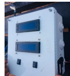
Fig -4 : Temperature recorder of the pyrolyzer prototype
