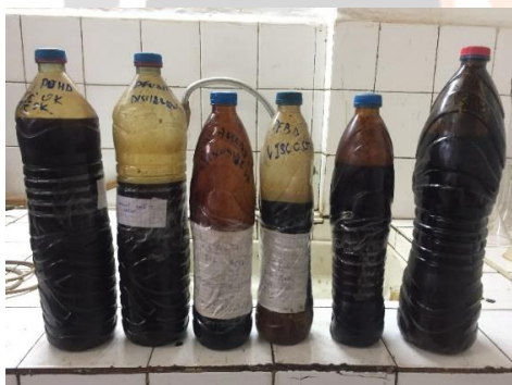
Fig -19 : Crude pyrolytic oils
