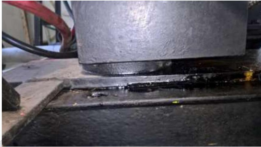
**Fig -3:** Elastomeric mounting
