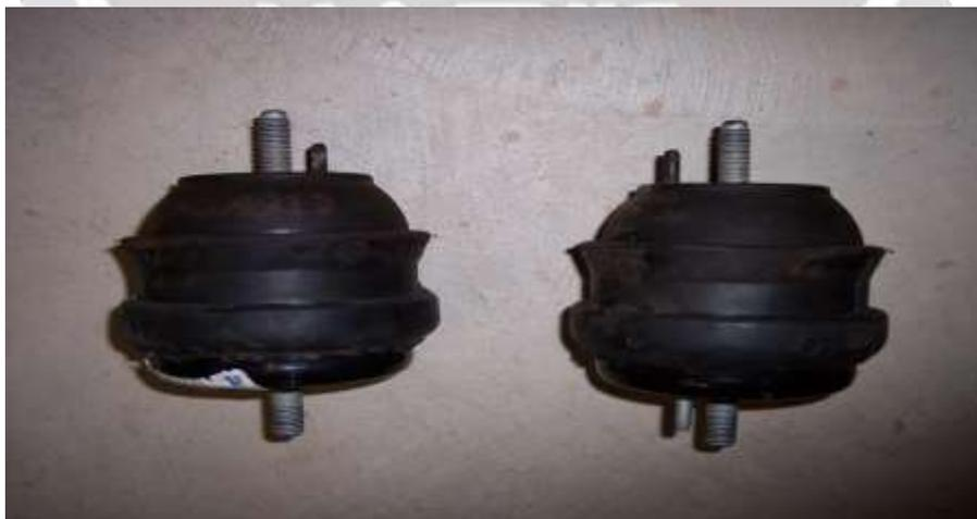
**Fig -4:** Passive Hydraulic Mount
