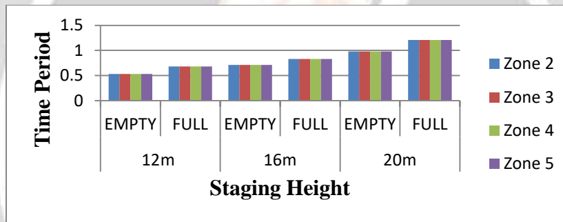
Fig 3.1: Time period v/s Different Staging for different zones and tank condition of water tank
