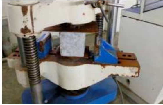
Compression Test On Cement Mortar
