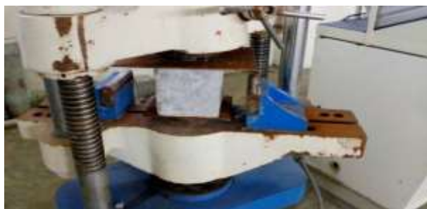
FIG.16 Compression Test On Concrete
