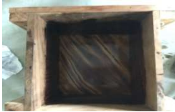
FIG. 3 PREPARED MOULD (30x30x30cm)
