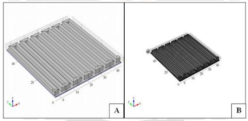
Fig-1: Serpentine flow field PEMFC (A) 3D model (B) Mesh model
