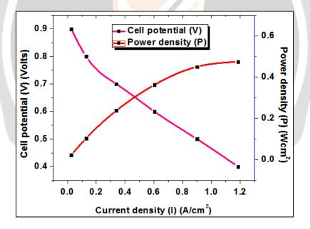
Fig-3: Power density and Polarization curves of all cell potentials
