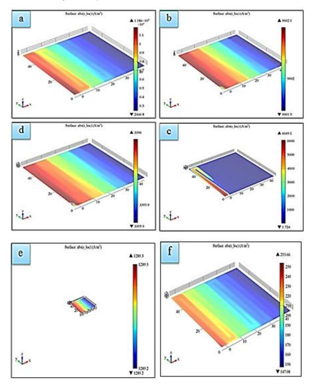
Fig-2: Current density of serpentine flow field PEMFC at cell potential (a) 0.4V (b) 0.5V (c) 0.6V (d) 0.7V (e) 0.8V (f) 0.9V
