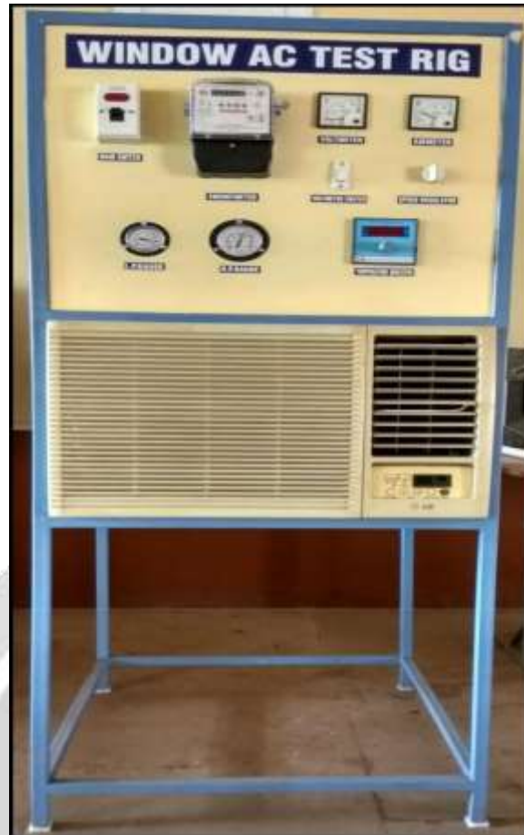
Fig.-2: Window Air Conditioning Test Rig 2.2 Refrigerant charging:
