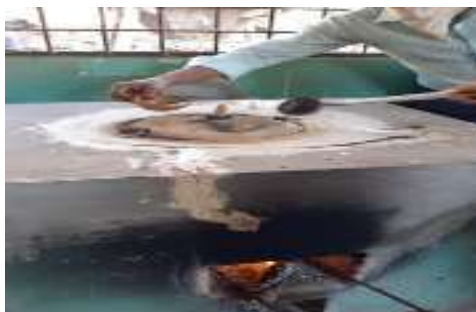
Fig-8 Removing the hot sand around the neck of the Kupi , which favours sublimation of Khageshwara Rasa around the inner side of bottle neck.
