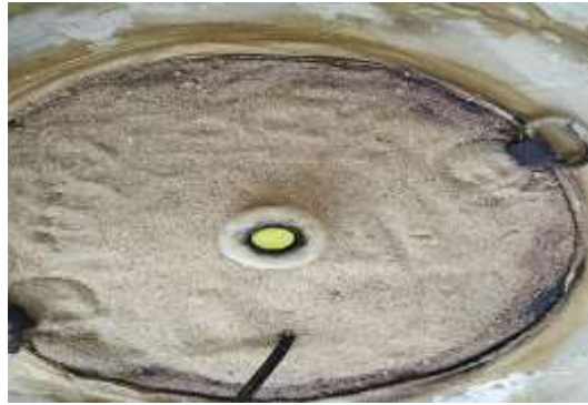
Fig-5 Yellow fumes inside the bottle, indicating melting of Gandhaka .
