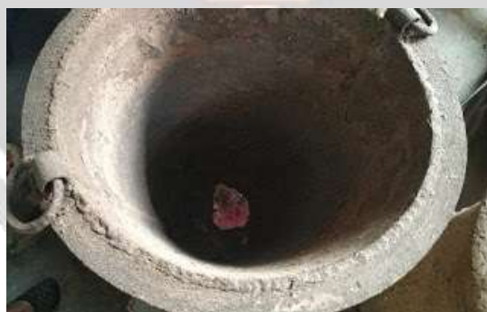
Fig-1 Valuka Yantra with Abhraka flakes at the centre. Abhraka is heat resistant and works as a mediator to transmit controlled heat to the sand, filled in the Valuka Yantra .
