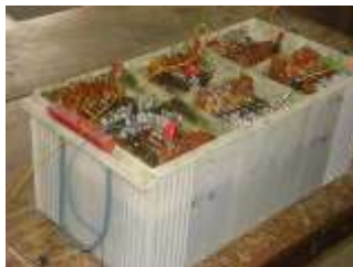
Figure-16: Experimental Setup of Cells of PKL.
