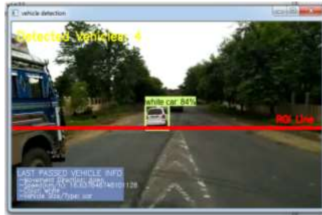
Fig. 4: System output. Text accompanying each detection gives the count, type, speed, direction and color of the vehicle.
