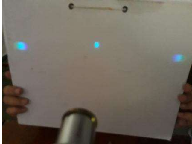
Fig -3: Diffraction of light emitted from LED
