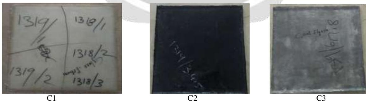
Fig 2: C1:without filler material C2:with coal powder C3:with fly-ash
