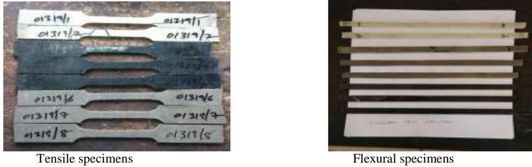
Fig 3: Dogbone shaped specimen after cutting according to ASTM standard
