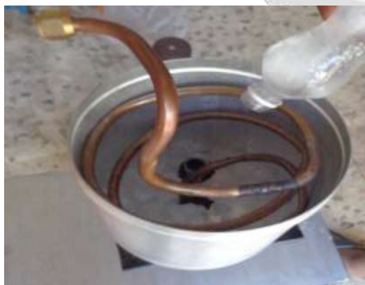
Final stage of condenser
