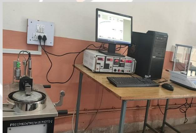
**Fig.3- Photograph of experimental set up (Tribometer TR-20LE)**
