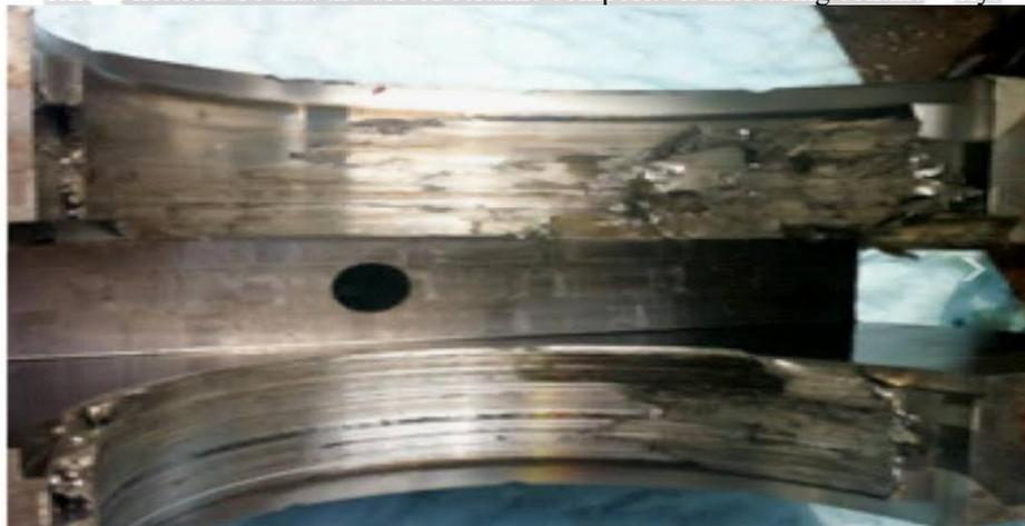
Fig 1- Failure Occurs in Sleeve bearing
